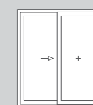
Two-part element with sliding door and fixed glazing unit
