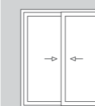
Two-part element with two sliding sashes
